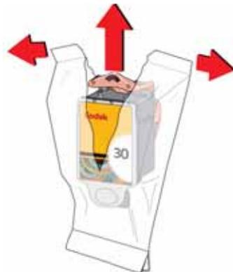
**IMPORTANT:** *To prevent the printhead from drying out, insert the ink cartridge into the printhead immediately.*
