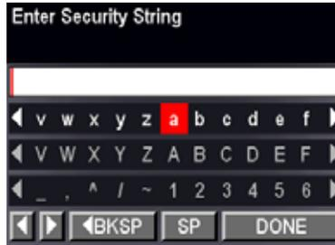
On the control panel, press ▲, ▼, ◀ or ▶ to select the letters and numbers, using the correct uppercase and lowercase letters. Press **OK** after each character. When you are done, select **DONE**, then press **OK**.
