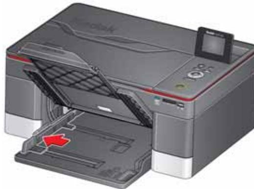
4. Fan and stack the paper, then insert it into the paper input tray.
