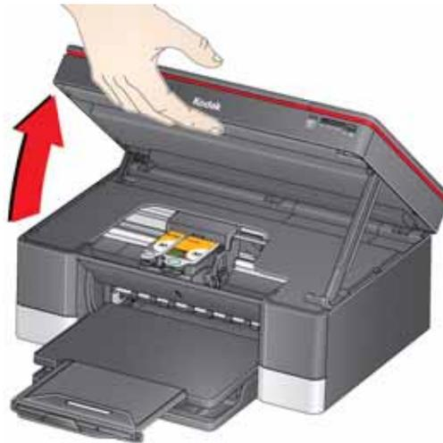
The ink cartridges are located in the printhead.
