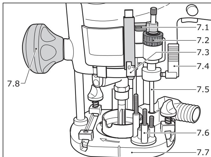
The milling depth is adjusted in three stages:
