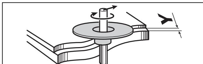
$$Y = 1/2 (\varnothing \text{ copying ring} - \varnothing \text{ cutter}) / 2$$
