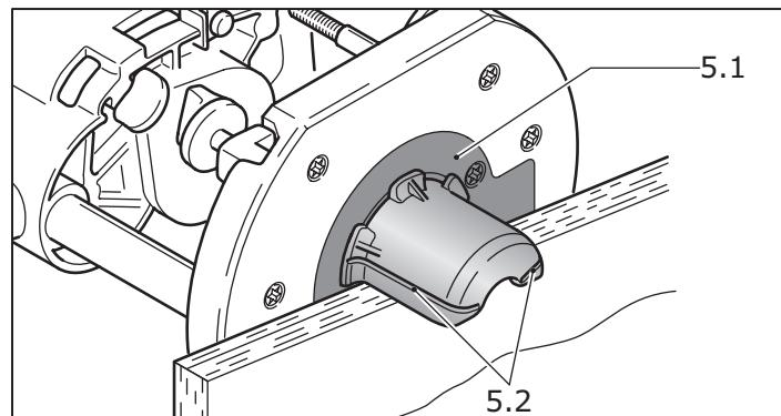
Using the KSF-OF chip catcher (sometimes included in the scope of delivery), the efficiency of the extraction can be increased when routing edges.
