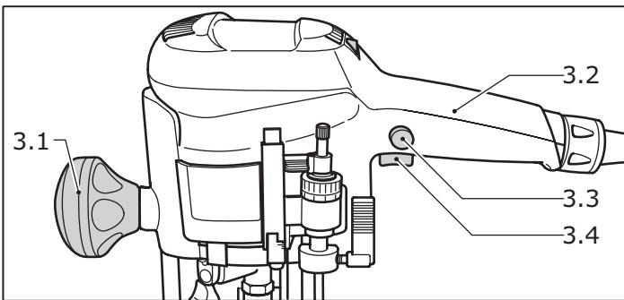
**WARNING** Keep the machine steady during switching and during use by holding the handle (3.2) and the additional handle (3.1) with both hands.
