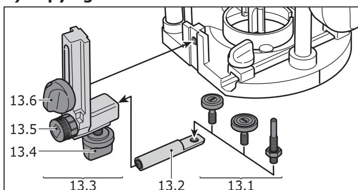
The angle arm WA-OF (13.3) and copier scanning set KT-OF, consisting of roller holder (13.2) and three copying rollers (13.1), are required for the copying device.
