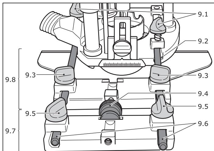
The parallel guide (9.8) (accessory) can be used for routing parallel to the edge of the workpiece.
