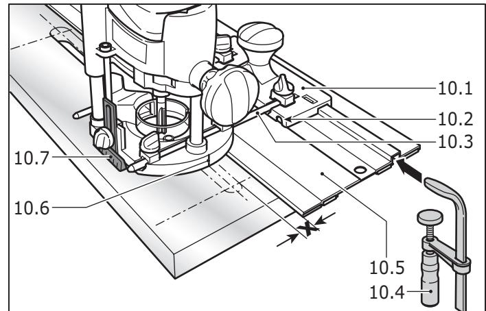
The guide system (accessory) facilitates routing straight grooves.
