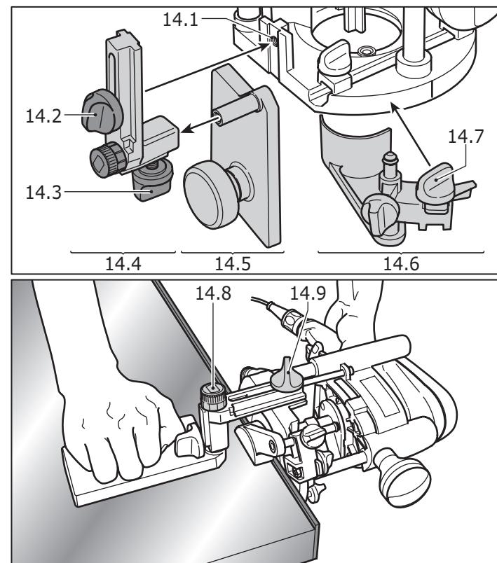
Protruding edge bands can be flush trimmed with the angle arm WA-OF (14.4) in connection with the guide plate UP-OF (14.5) (accessories).
