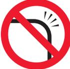
**CAUTION! Do not sharply bend the cable; the cable will be damaged if severely bent.**
