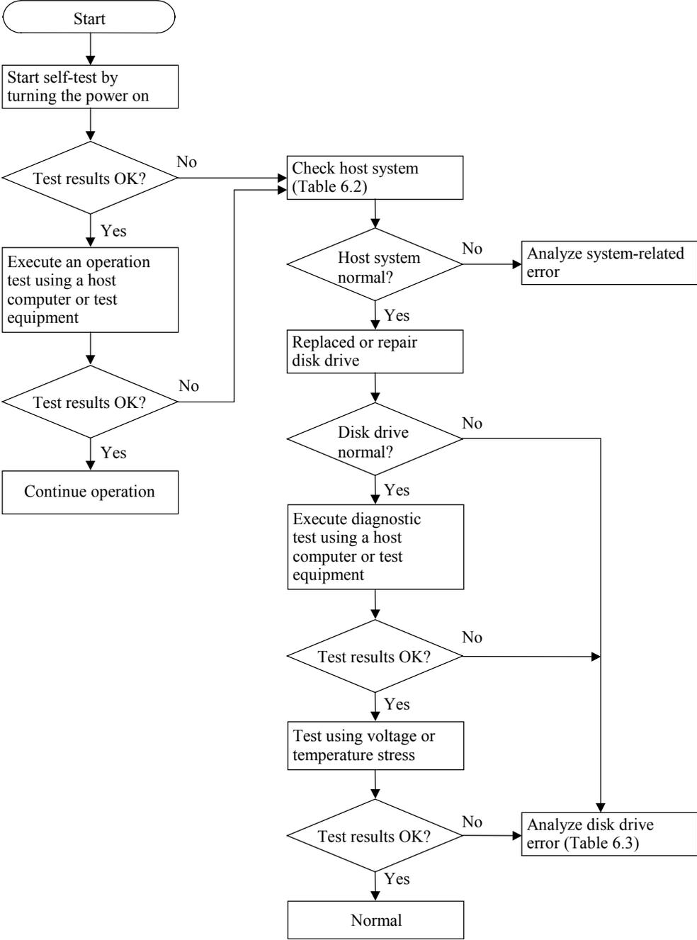
Figure 6.3 Test flowchart
