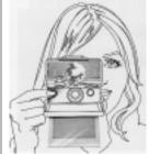
Look through the center of the eyepiece. Rest your thumb on the back of the shutter housing, with your right forefinger on the shutter button. Curl the other fingers into your palm.
