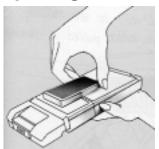
Hold the camera in the palm of your left hand. Grasp the sides of the viewfinder cap at the rear (ribbed surfaces).
