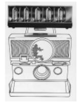
the way as FlashBar is inserted, then release it slowly.) On other models, the FlashBar socket is on the top front of the camera body above the lens or sonar.
