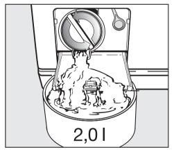
Unscrew the fluff filter lid until water runs out.
