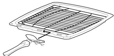
Slide the handle to the left and over the central bump on the grill pan.
