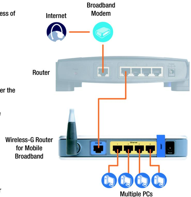
Figure 4-6: Diagram for Connection to Another Router
