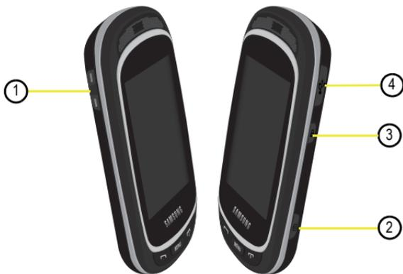
1. **Volume keys** allow you to adjust the ringer volume in standby mode or adjust the voice volume during a call. When receiving an incoming call, pressing the volume key mutes the ring tone. Press and hold the volume key to reject a call.
