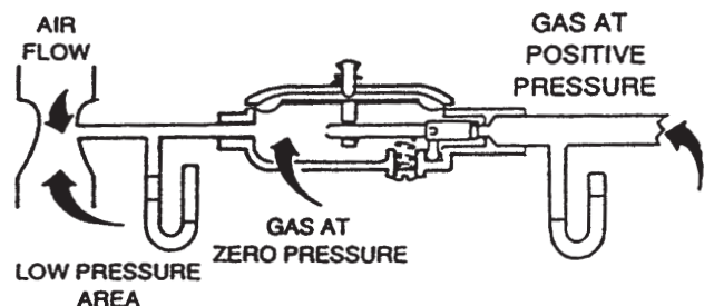
Figure 2.16 – LP Gas Carburetion Diagram
