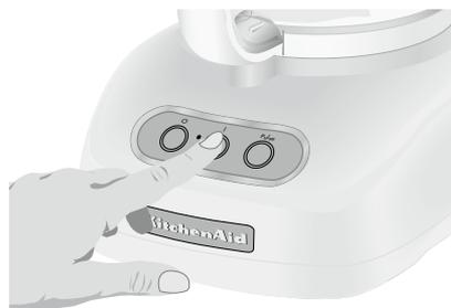
2. To stop the Food Processor, press the "O" Button. The indicator light will go out and an automatic brake will stop the action of the blade within seconds.
