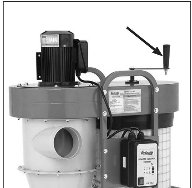
**Figure 38.** Brush handles for cleaning canister filters.
