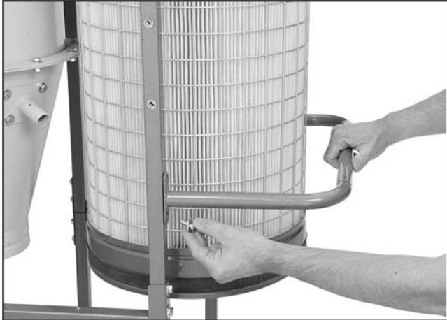
**Figure 11.** Installing the hand rail.
