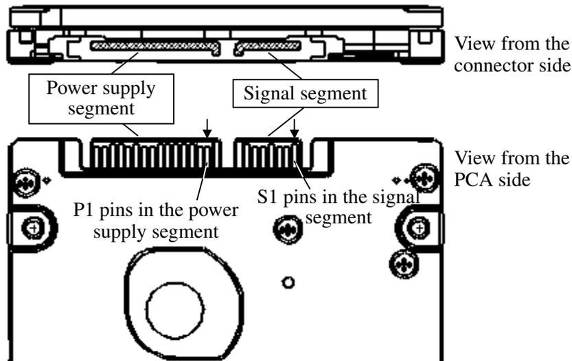
**Figure 3.8 Power supply pins (CN1)**
