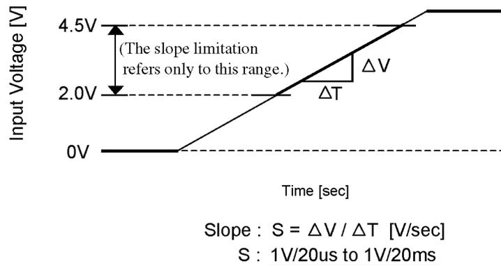
**Figure 1.1 Permissible range of +5V rise slope**
