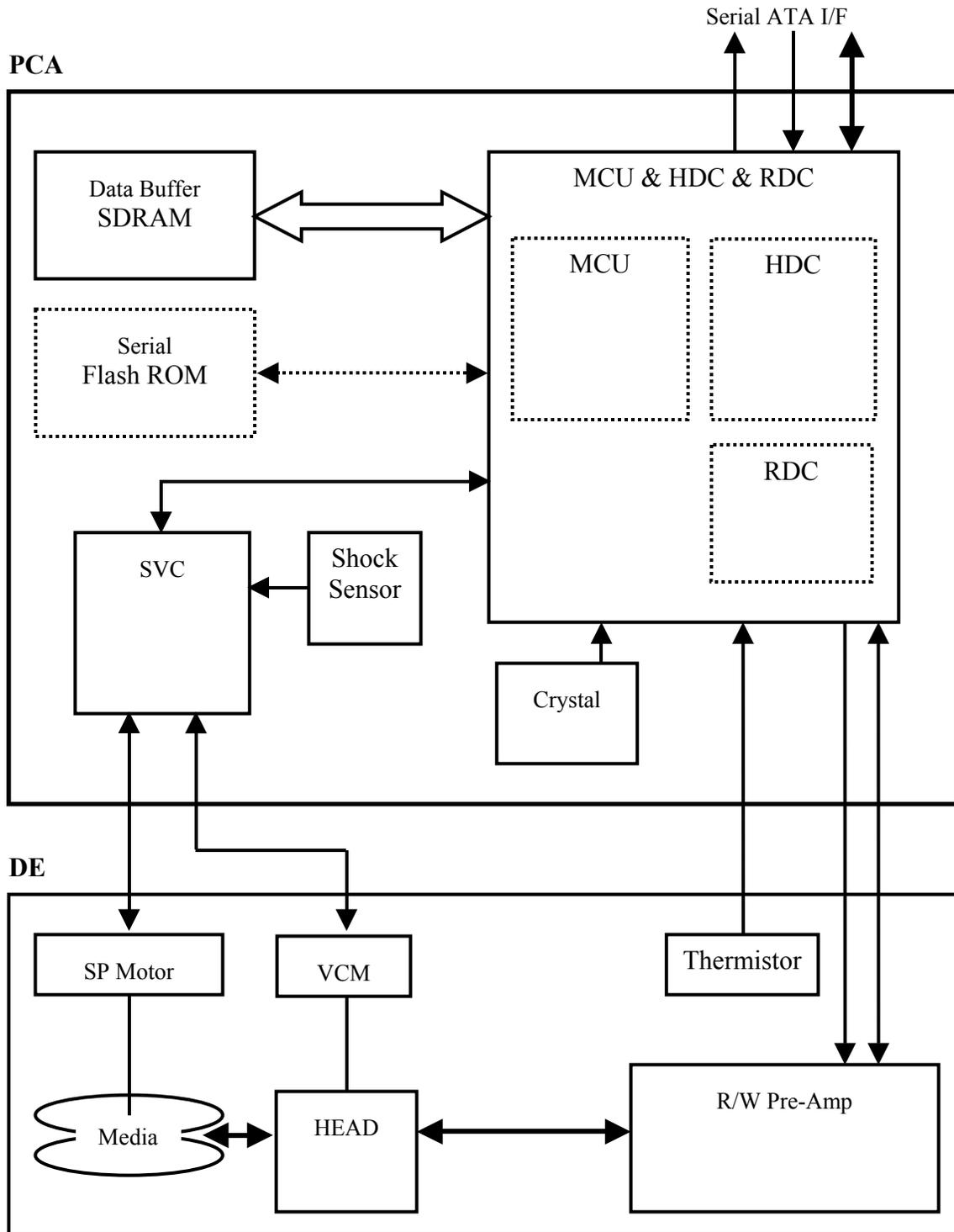
Figure 4.2 Circuit configuration
