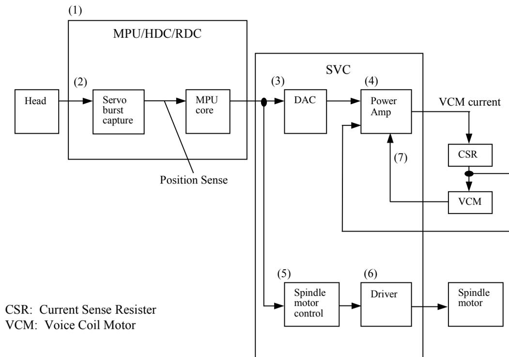
**Figure 4.6 Block diagram of servo control circuit**
