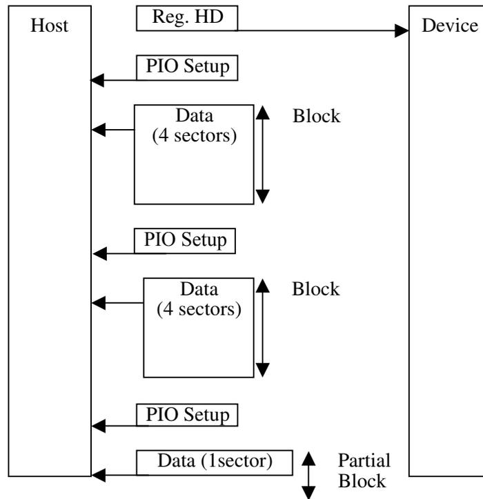
**Figure 5.12 Execution example of READ MULTIPLE command**
