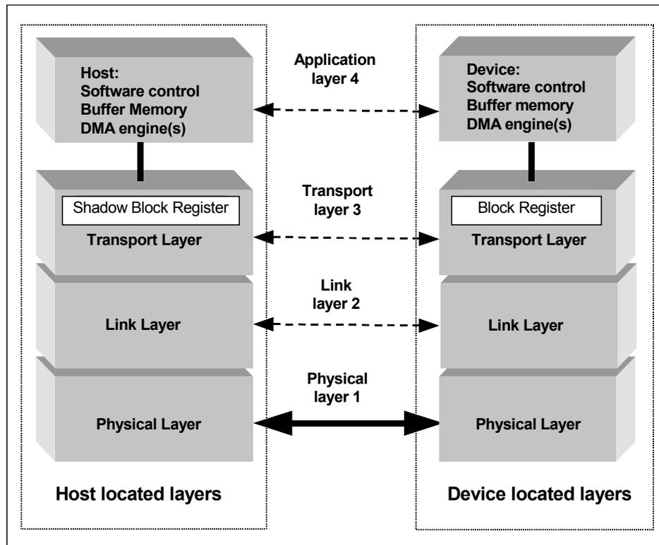
Figure 5.3 Conceptual diagram of communication layers
