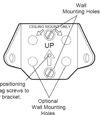
The nail hole is for positioning only. You must use lag screws to mount the header bracket.
