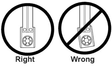
When tightening the screws, be sure to keep bracket parallel to the rail. Otherwise, the rail may bow when opener is operated.
