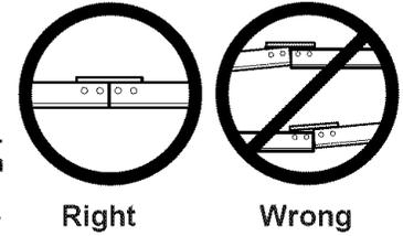
If T-rail is not assembled EXACTLY as shown, trolley will not travel smoothly along length of rail or it will hit against the nuts.
