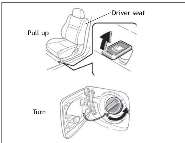
**NOTE:** If the cap is not tightened enough, Check Engine "CHECK" indicator may illuminate.
