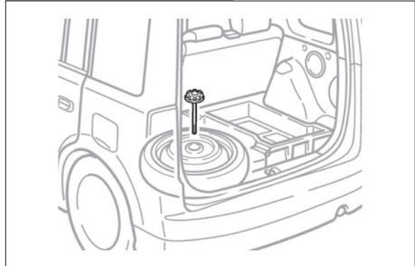
Loosen the bolt and remove it.
