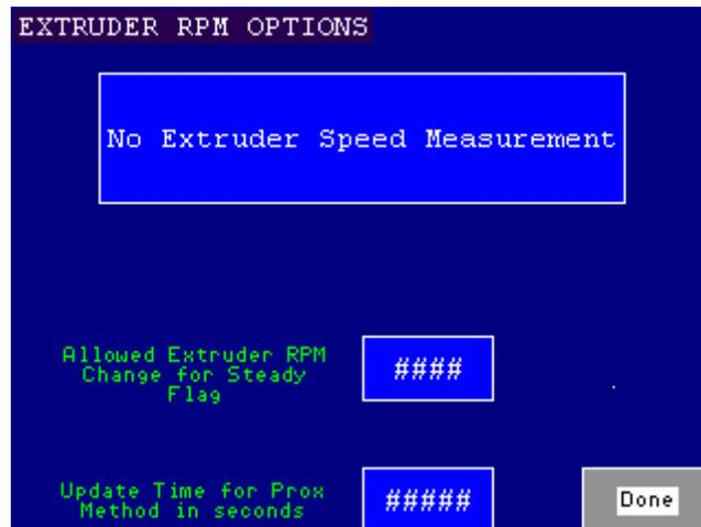
This gives you the option of having no extruder speed input, writing the extruder speed to the blender through the Ethernet, or using a proximity sensor on the end of the extruder screw.
