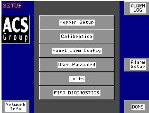
Select “Mass Flow FIFO Data” or “Feeder FIFO Data”
