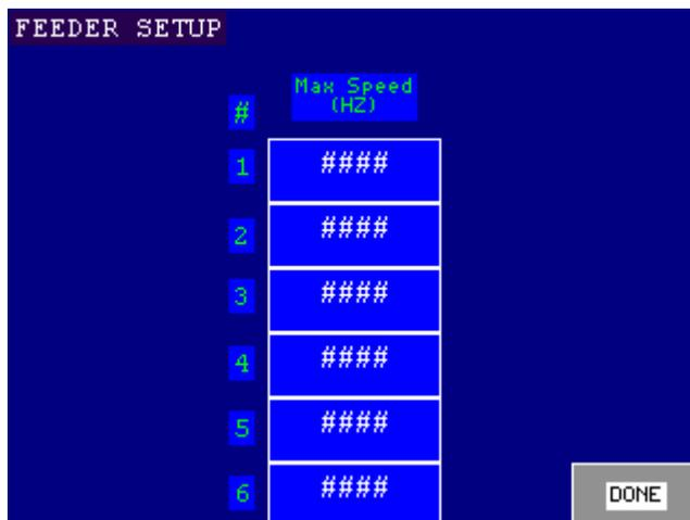
This screen allows you to enter the maximum auger speed in Hertz.
