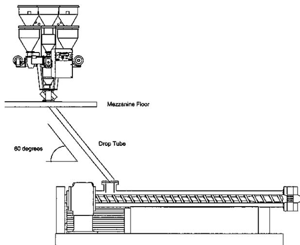
*Note: Ensure that the feed tube angle is steep enough (60 degrees is recommended).*
