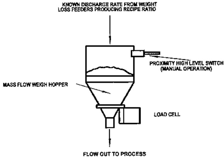
*Note: The lower or common mass flow weigh hopper uses the change in weight over time, of material contained in the hopper over time to calculate its discharge rate (differential rate). This learned discharge rate is then summed with the known total metering rates of the blender feeders to learn the actual processing rate of the processing machine. The blender output rate is then adjusted to match the learned processing rate, eliminating the need for a blender mixer.*
