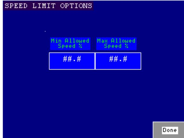
This allows you to set the minimum and maximum speed for the motor drives as a percentage. The drives are not supposed to be run at less than 8 hertz and should not be run above 115 hertz.
