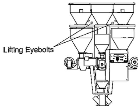
**Caution!** *Remove hoppers if necessary to prevent damage.*
