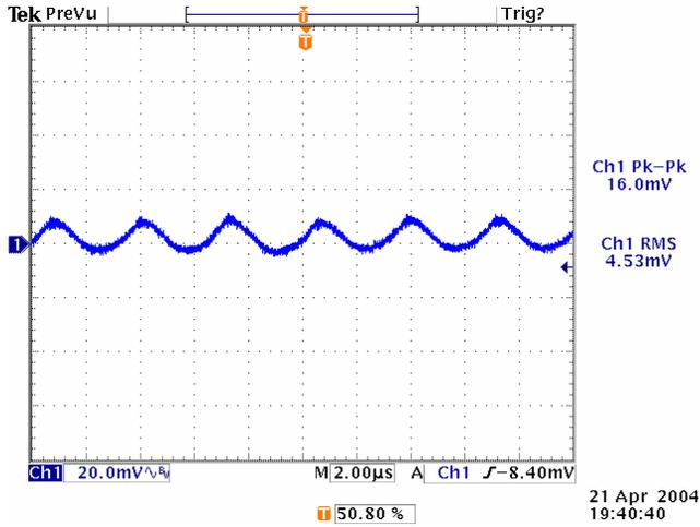
Figure 7: Output ripple & noise at 3.3Vin, 2.5V/10A out
