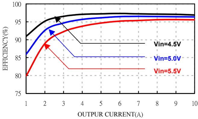
Figure 1: Converter efficiency vs. output current (3.3V out)
