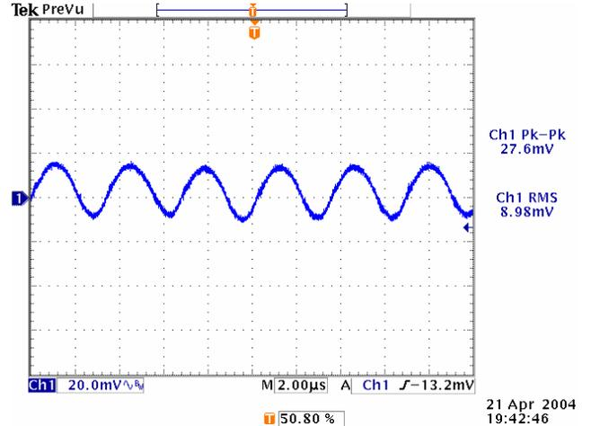
Figure 10: Output ripple & noise at 5Vin, 1.8V/10A out
