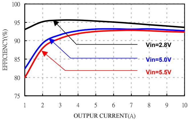
Figure 3: Converter efficiency vs. output current (1.8V out)
