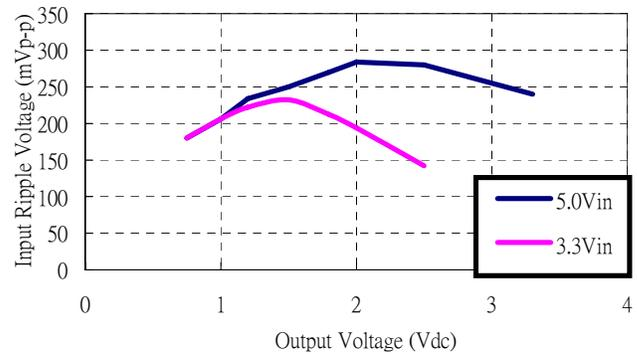
**Figure 32:** Input voltage ripple for various output models, IO = 10 A (CIN = 2x100 µF tantalum // 47 µF ceramic)
