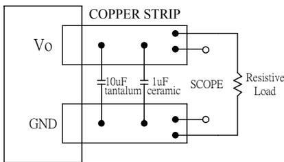
Note: Use a 10µF tantalum and 1µF capacitor. Scope measurement should be made using a BNC cable.
