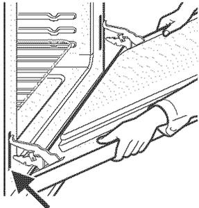
HINGE SLOT - Door removed
