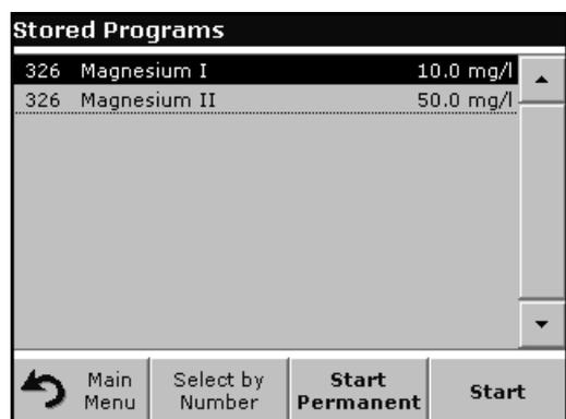
Some tests can be used for different measuring ranges. After the sample cuvette/vial has been inserted, a list of the different measuring ranges is displayed.
