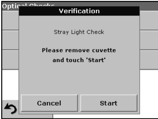
7. Remove any cuvettes/cells from the cell compartment and press **Start**.
