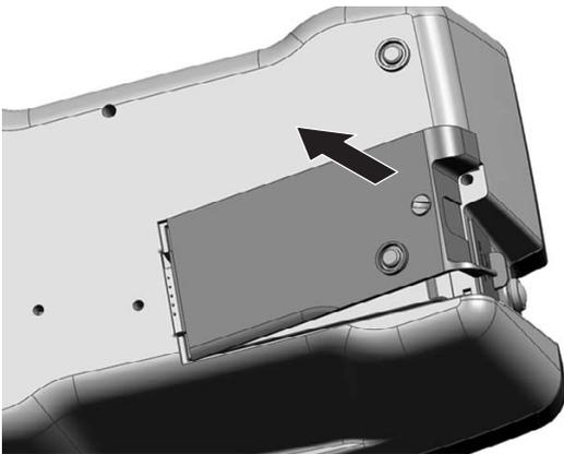
8. Use a screwdriver (slotted or cross-headed) to remove the screws from the lamp fitting.
