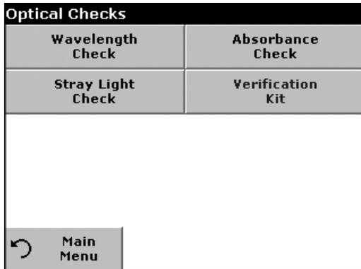
1. Press **Optical Checks** in the System Checks menu.
