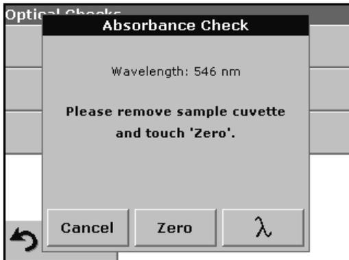
The Absorbance Check test is used to test the photometric accuracy and repeatability of the instrument.
