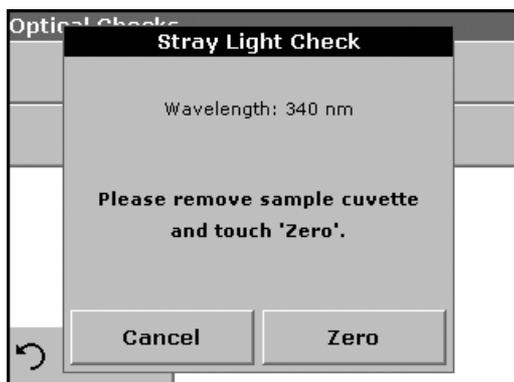
1. Press **Stray Light Check** in the Optical Checks menu.
