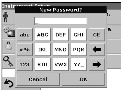
3. Use the alphanumeric keypad to enter a new Password (up to 10 characters each) and press **OK** to confirm.
