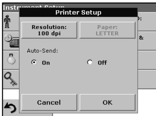
4. Select **Auto-Send: On** to send all measured data automatically to the Thermal printer.
