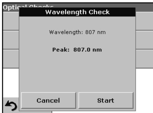
3. The result is displayed and is to be compared with the nominal/standard data (given in the quality control certificate) of the sample cuvette/cell.
