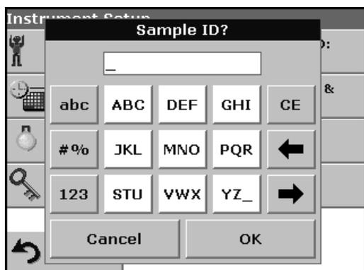
This display is used to enter letters, numbers and symbols as needed when programming the instrument. Unavailable options are disabled (grayed out). The icons on the right and left of the screen are described in Table 1.
