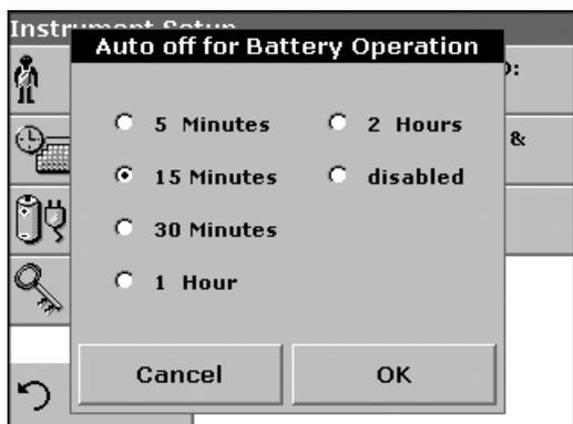
3. Select one of the options under **Auto off** to set the length of the idle period that can elapse before the instrument automatically switches off when running on battery power.
