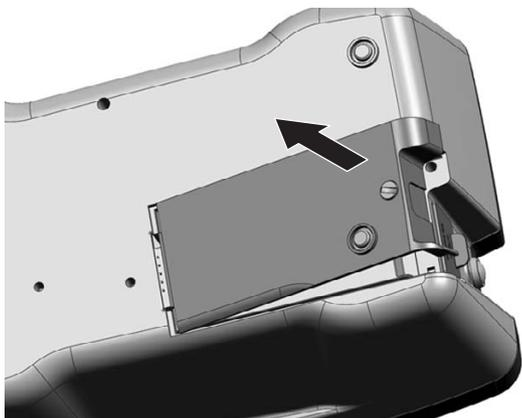
5. Use a screwdriver or a coin to remove the screw from the cover.
