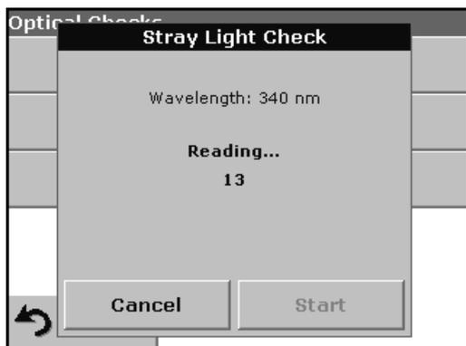
4. Insert the sample cuvette/cell or reference filter into the cell compartment #2. Close the cell compartment. Press **Start**.
