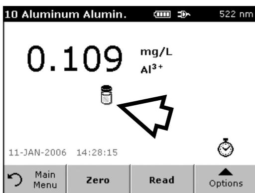
*Note: The reagent blank icon is shown in the result display (see arrow) when the function is active.*
