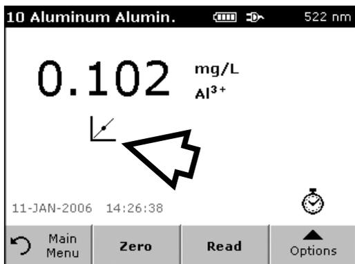
5. Press **Adjust** to enable the Standard Adjust. The Standard Adjust icon will appear.
