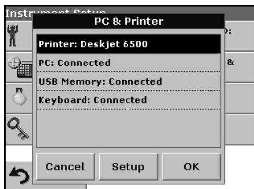
1. Press **PC & Printer** in the Instrument Setup.
