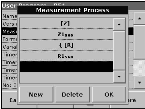
**Deleting an element of a measuring sequence**
