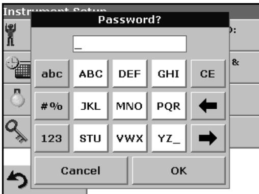
1. Press **Password** in the Instrument Setup.
