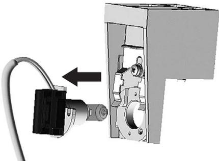
12. Remove the halogen lamp complete with the plug panel.
