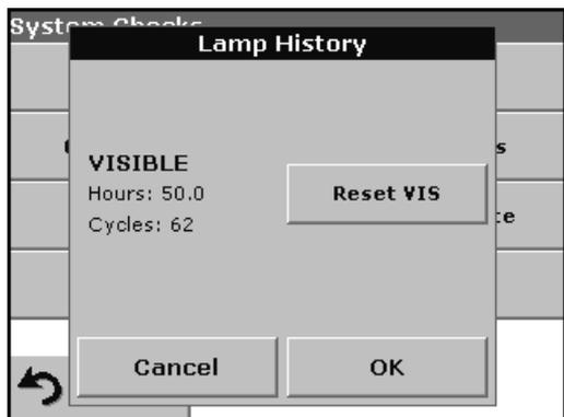
After a lamp is replaced and the Lamp History is reset, the display of the total operating time is reset to 0.
