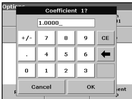
3. To change a wavelength, press one of the "λx:" keys. Enter the desired wavelength coefficient into the numeric keypad. Press **OK** to confirm.
