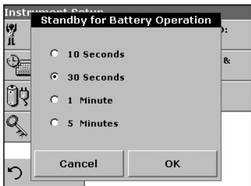
2. Select one of the options under **Standby mode** to set the length of the idle period that can elapse before the instrument switches to the Standby mode when running on battery power.
