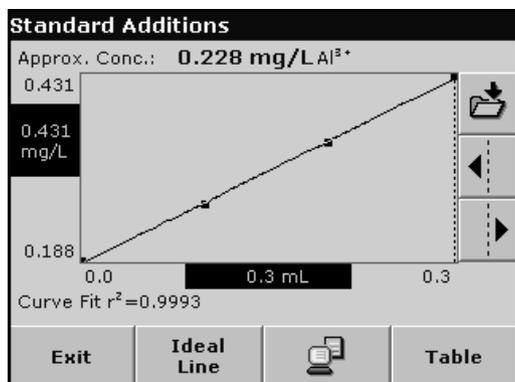
11. After all the standard addition solutions have been measured, press **Graph**.
