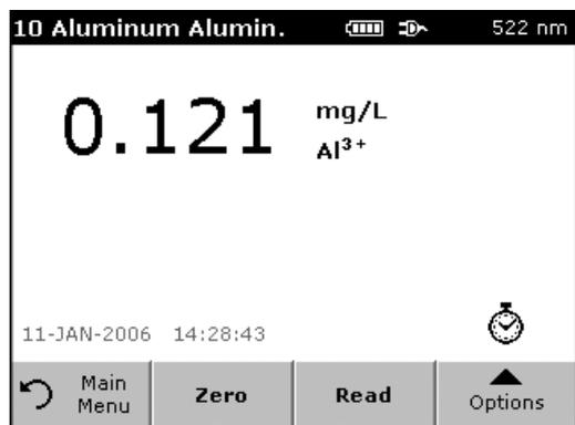
4. Remove zero solution and insert sample cuvette/cell into the cell compartment.
