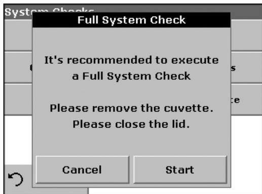
If the instrument detects any deviation relative to the last calibration, a system check has to be carried out.
