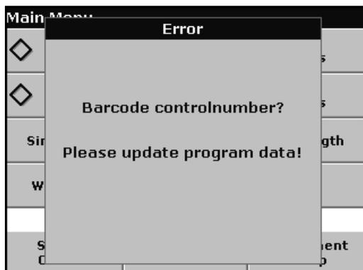
Using the data provided in the barcode, the instrument automatically sets the measurement wavelength and factors. If a discrepancy is detected between the barcode data and the stored data or a new test is identified, the instrument requests an update.
