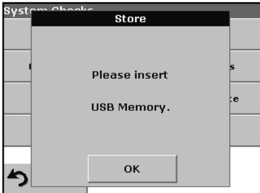
**Note:** If the USB stick is not connected, the message "Please insert USB Memory" is displayed. Connect a USB stick, in order to store the data. Press **OK** to confirm and press **Store** again.
