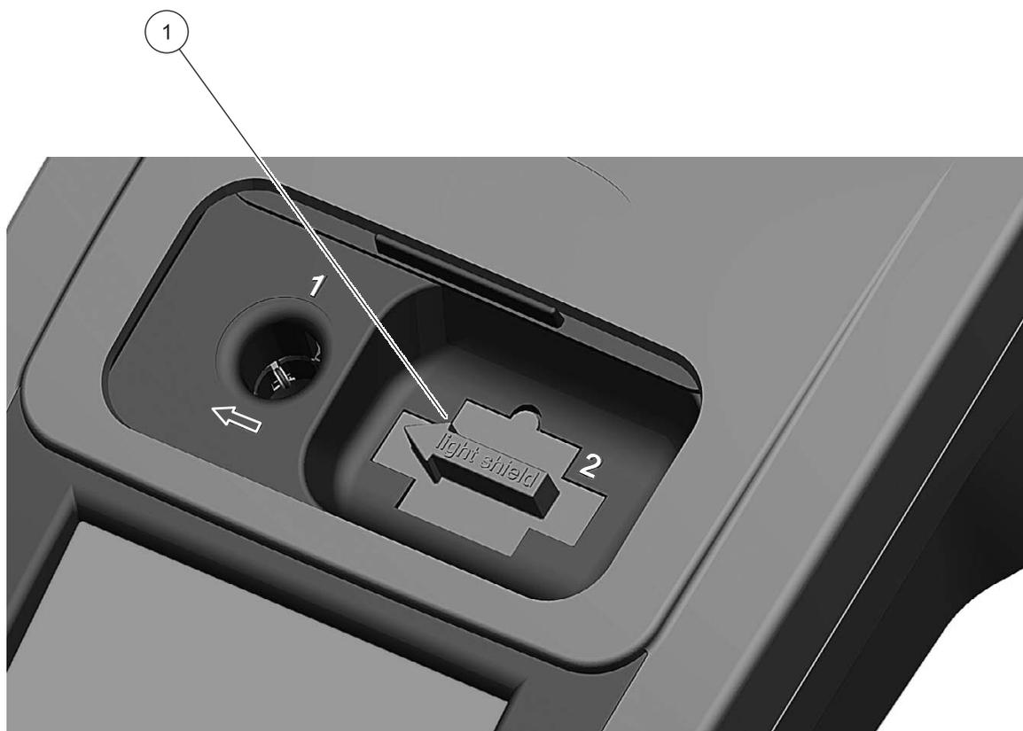
Figure 7 Light Shield in place
