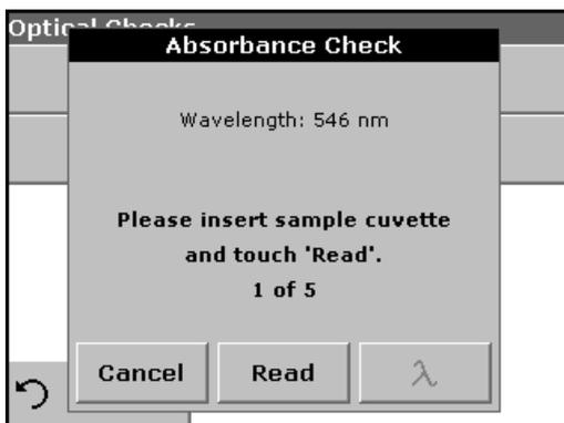
5. Insert sample cuvette/cell into the cell compartment and press **Read**.
