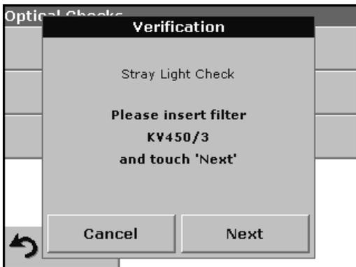
8. Insert the different filter in the given order one after the other. Press **Next** after inserting a filter.
