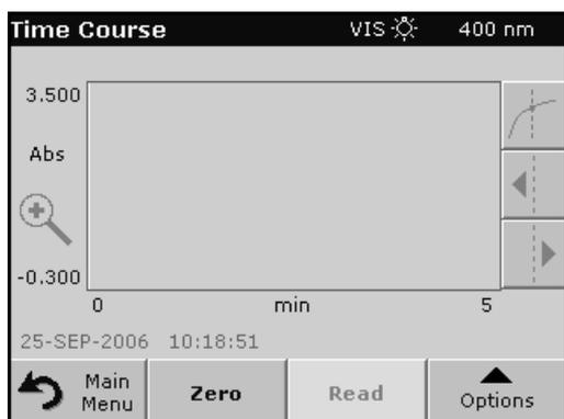
After the parameters have been selected, the instrument must be blanked, then the sample can be analyzed.
