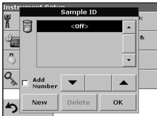
1. Press **Sample ID** in the Instrument Setup.
