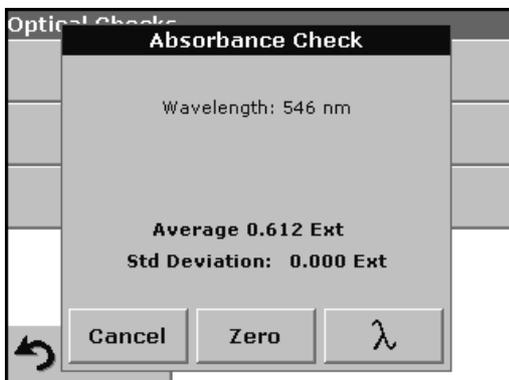
7. The result is displayed and is to be compared with the nominal/standard data of the sample cuvette/cell.
