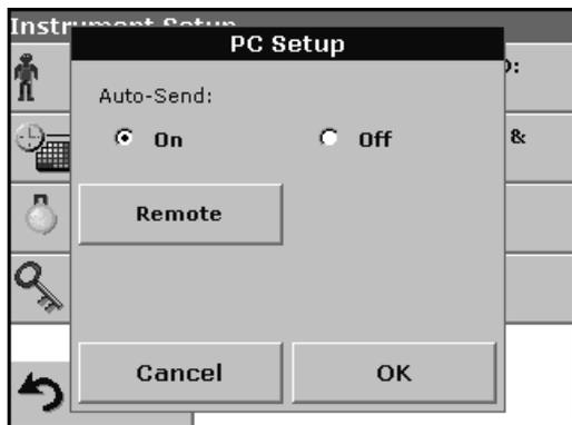
4. Select **Auto-Send: On** to send all measured data automatically to the PC.
