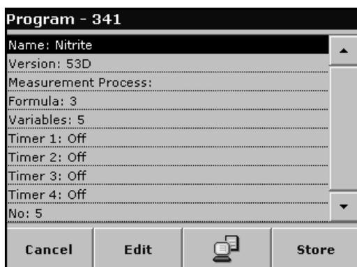
3. After "Program not available", a data overview is displayed, including the specifications of the test that is to be revised.
