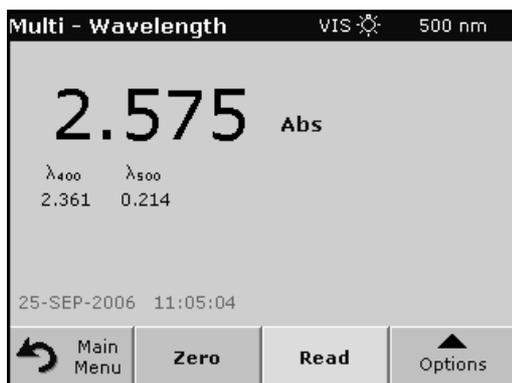
1. Insert the blank cuvette/cell into the cuvette/sample cell holder. Press **Zero**.
