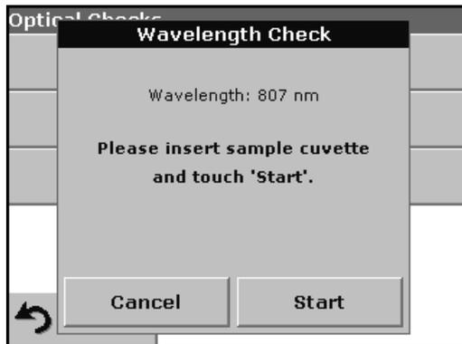
1. Press **Wavelength Check** in the Optical Checks menu.
