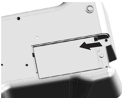
8. Push in the battery so that the contacts of the instrument can be plugged into the socket of the battery.
