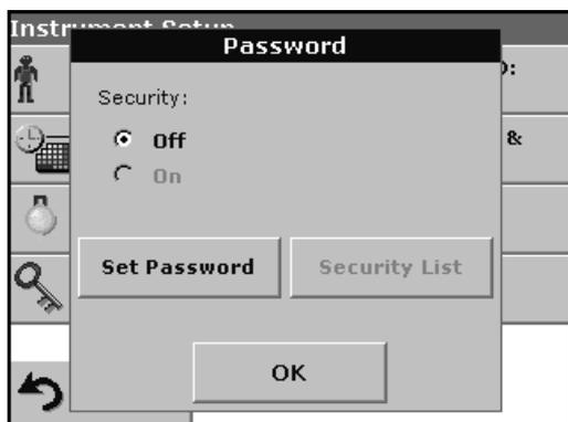
1. Press **Password** in the Instrument Setup menu.
