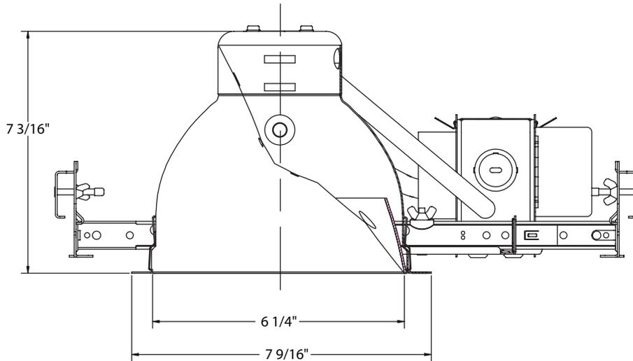
Complete Fixture consists of Frame-In Kit and Reflector Trim. Select each separately.
