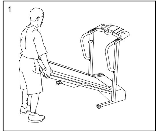
2. Move your right hand to the position shown and hold the treadmill firmly. Press out on the storage latch. Raise the treadmill until the storage latch closes over the catch. **Make sure that the storage latch is fully engaged over the catch.**
