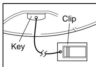
Insert the key fully into the console. After a moment, the displays will light. **Test the clip by carefully taking a few steps backward until the key is pulled from the console. If the key is not pulled from the console, adjust the position of the clip.**
