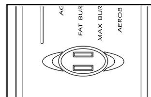
**your thumb will be restricted and your pulse will not be detected.** After a few seconds, the heart-shaped indicator in the Fat Calories/Calories/Pulse display will begin to flash, one or two dashes (—) will appear, and then your heart rate will be shown. Hold your thumb on the heart rate sensor for about 15 seconds for the most accurate reading.
