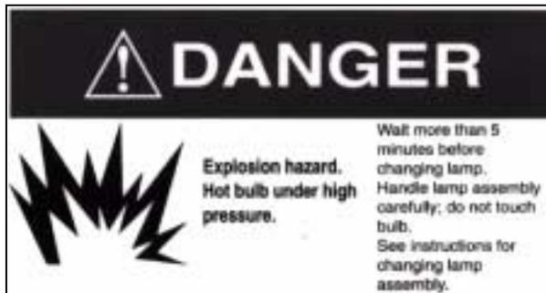
*Explosion hazard. Hot bulb under high pressure. Wait more than 5 minutes before changing lamp. Handle lamp assembly carefully; do not touch bulb. See instructions for changing lamp assembly.*
