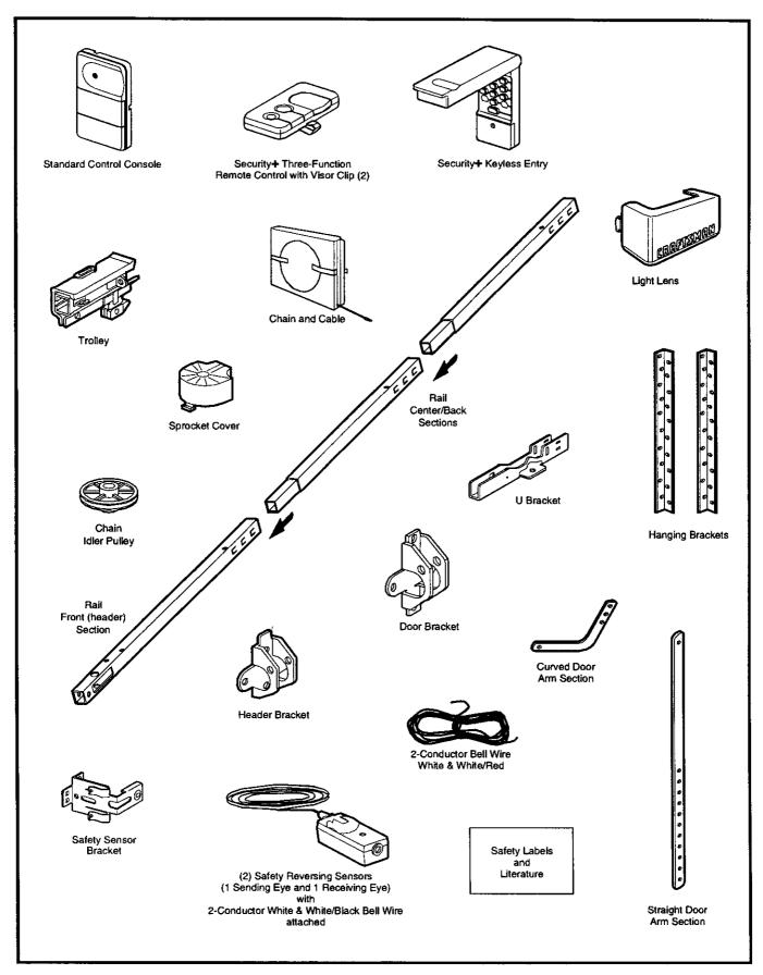
Separate all hardware from the packages in the rail carton and the opener carton, as shown below, for the assembly and installation procedures.
