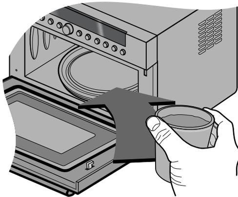
**6** Press the **STOP/CLEAR** button, and press the **START** button one time to set 30 seconds of cooking time.
