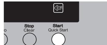
During **Quick Start** cooking, you can extend the cooking time up to 9 minutes 59 seconds by repeatedly pressing the **Quick Start** button or by using **DIAL**.
