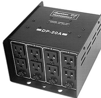
Now with a new case design and 2 plugs per channel, the DP-20A™ has all the same features of the DP-20™ by American DJ™. The DP-20A™ is a 0-10V analog, 4 Channel, 15A max, 600W per channel dimming power pack. Each channel includes warm-up feature, take out,
