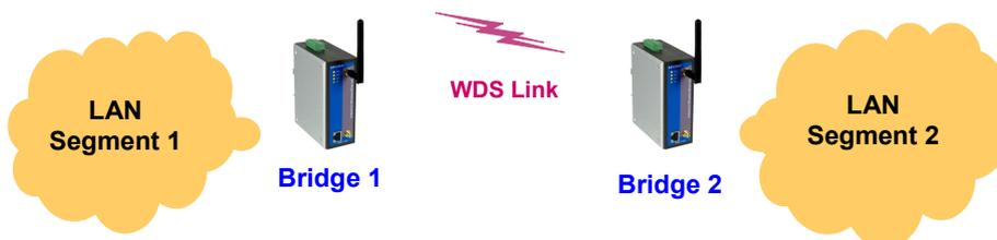
By WDS, two or more LAN segments can be connected wirelessly. As illustrated in the above figure, a pair of wireless LAN-to-LAN bridges is used to connect two LAN segments. Since the AP is WDS-enabled, it can be used as a wireless bridge.
