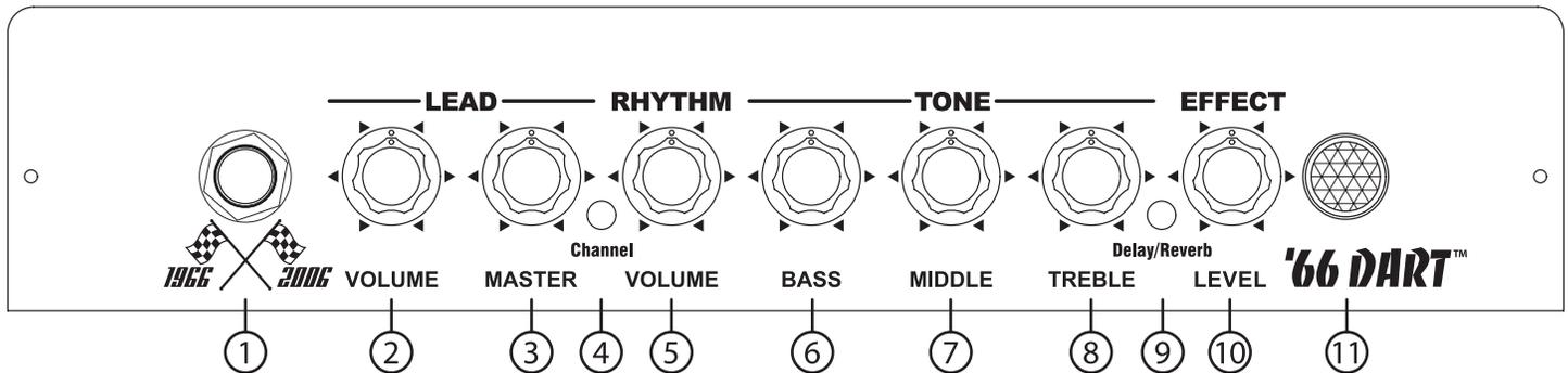
**1.) Guitar Input Jack** - This is a 1/4" 2-conductor input jack for plugging in your instrument. It is intended for guitars but will accept other instruments as well.
