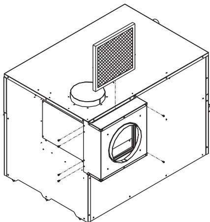
**Figure 24 – Attaching DV Box Adapter to Unit**
