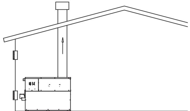
Figure 7 – Outside Combustion Air - Two Openings
