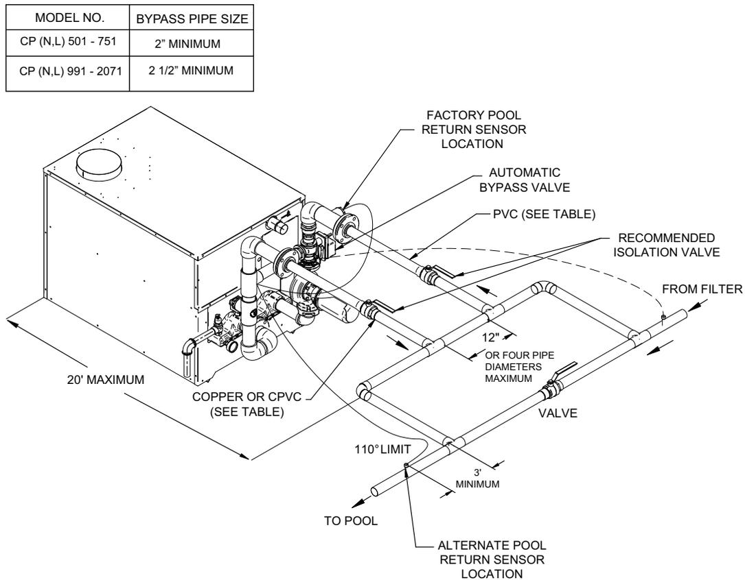
**Figure 35 - Heater is Beyond 15 Feet of Pool Piping**
