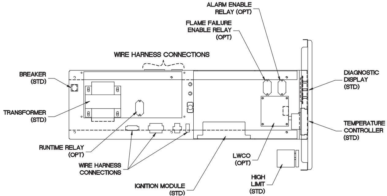
Figure 39 - Control Panel Component Location Drawing
