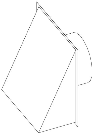
**Figure 15 – Air Inlet Cap for Sidewall Termination**
