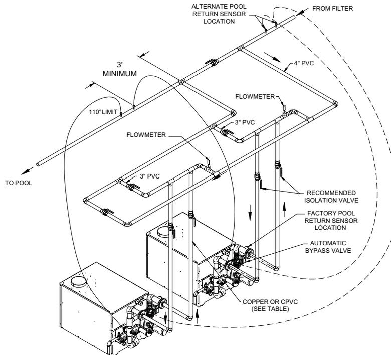
**Figure 37 - Heaters are Beyond 15 feet of Pool Piping**
