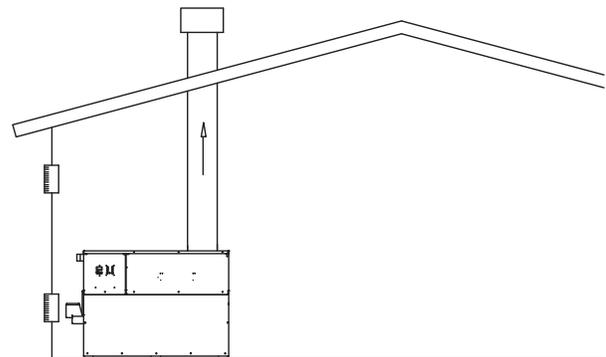
**Figure 17 – Conventional Negative Draft Vertical Venting with Combustion Air Louvers**
