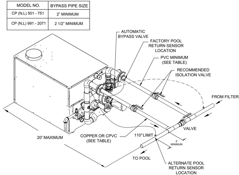
**Figure 34 - Heater is Within 15 Feet of Pool Piping**
