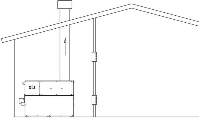
Figure 8 – Outside Combustion Air Through Ducts
