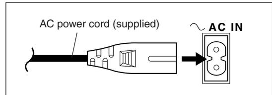
**Connect the AC power cord to the AC IN connector and a wall outlet.**
