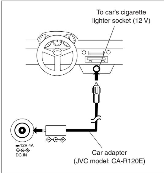
Connect a car adapter to the DC IN (12 V, 4 A) connector and the cigarette lighter socket.
