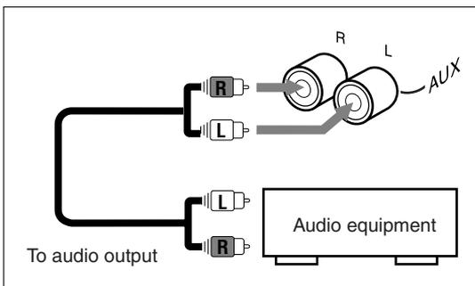
**For playing other equipment through this unit**, connect between the audio output jacks on the other equipment and AUX jacks by using audio cords (not supplied).
