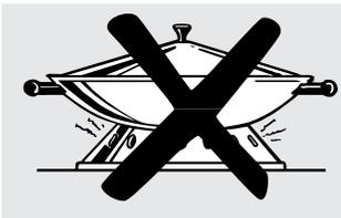
Do not use a round-bottomed wok on a support ring. Placing the ring over the burner or grate may cause the burner to work improperly, resulting in carbon monoxide levels above allowable standards. This could be dangerous to your health.
