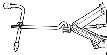
**Be sure to place the jack away from the rear edge of the rocker to avoid damaging the rear tire spoiler (pictured).**
