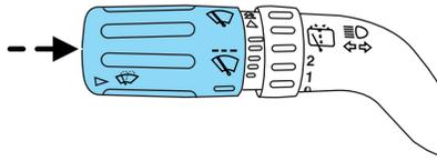
**Courtesy wipe feature:** One extra wipe will occur a few seconds after washing the front window to clear any excess washer fluid remaining on the windshield.
