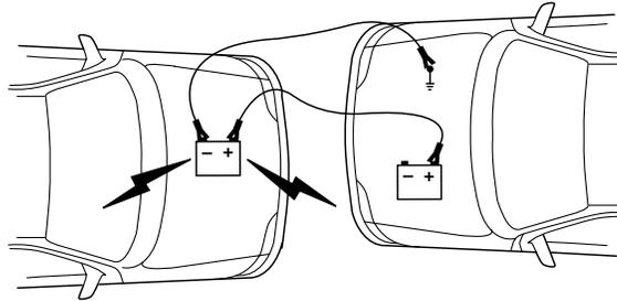
4. Make the final connection of the negative (-) cable to an exposed metal part of the stalled vehicle's engine, away from the battery and the carburetor/fuel injection system.
