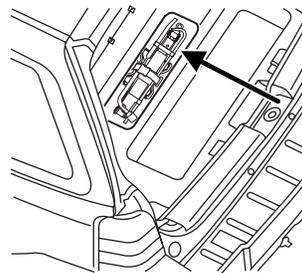
Unbuckle the strap and remove the jack and tools by pulling the right side up first. Remove the tools from the jack in order to remove the spare tire from under the vehicle.
