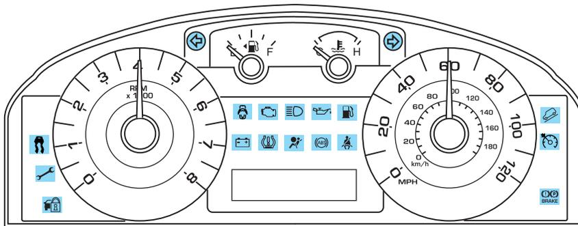
Warning lights and gauges can alert you to a vehicle condition that may become serious enough to cause extensive repairs. A warning light may illuminate when a problem exists with one of your vehicle's functions. Many lights will illuminate when you start your vehicle to make sure the
