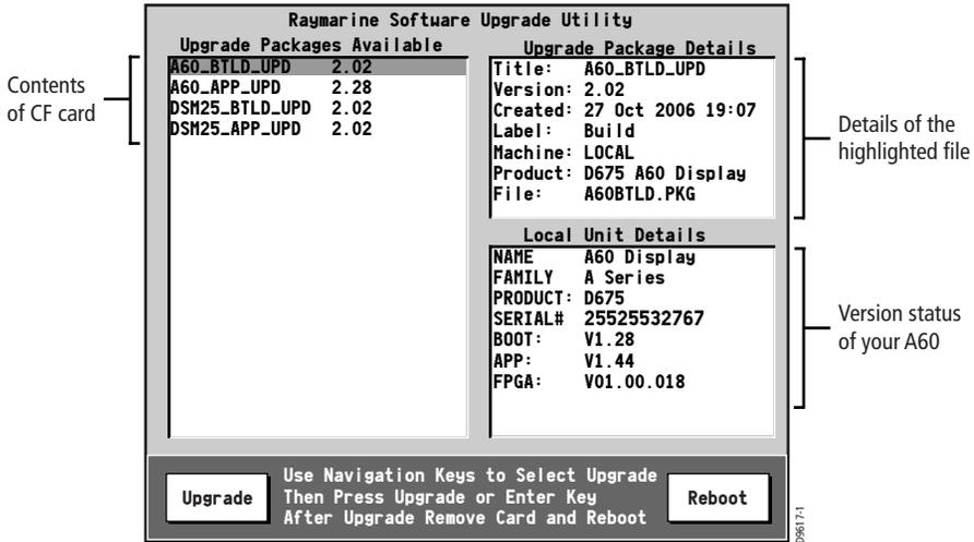
8. Compare the upgrades that are available in the Upgrade Packages Available field with the version displayed in Local Unit Details. If a newer version is available under Upgrade Packages Available, use the trackpad to highlight that file.
