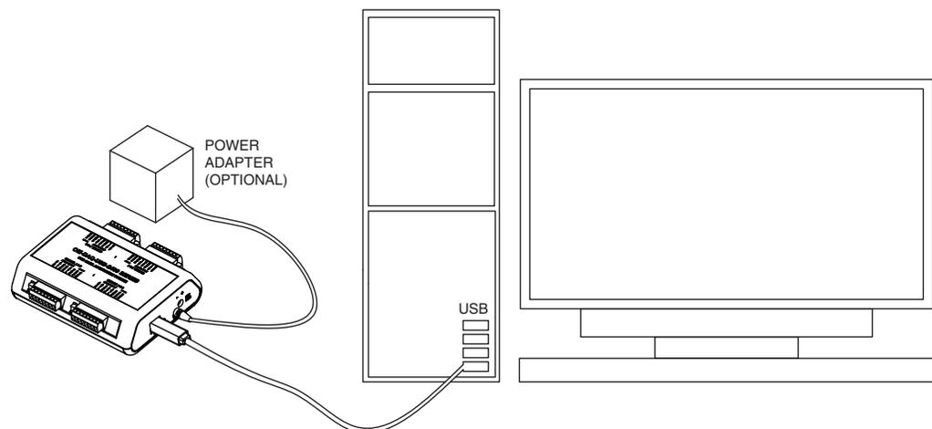
Figure 3-3. Direct Connection to a Computer USB Port(s)
