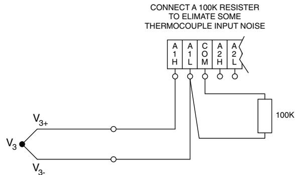
Figure 4-28. Thermocouple Wiring
