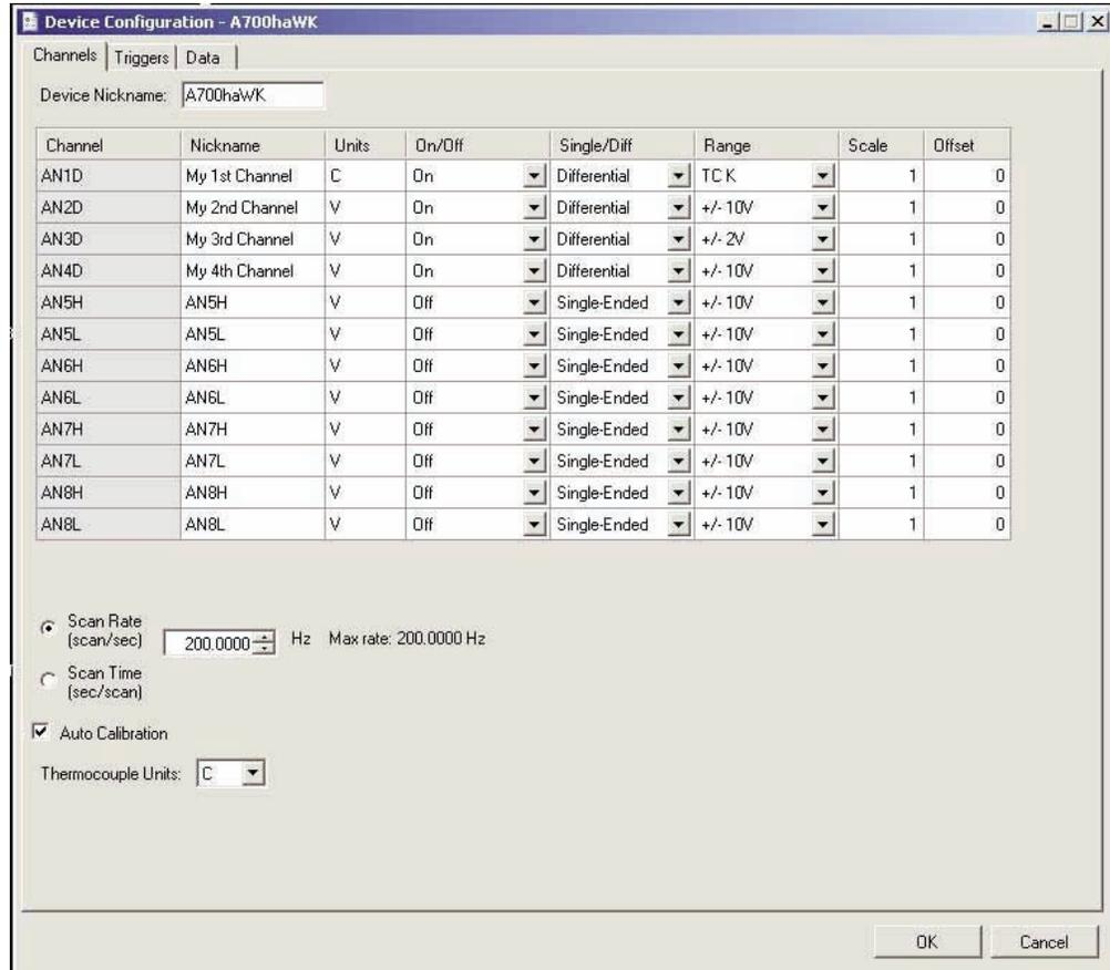
Figure 4-9. Configuration Mode - Channels Tab Screen
