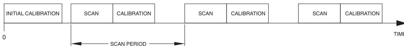
Figure 4-27. Calibration/Scan Arrangement
