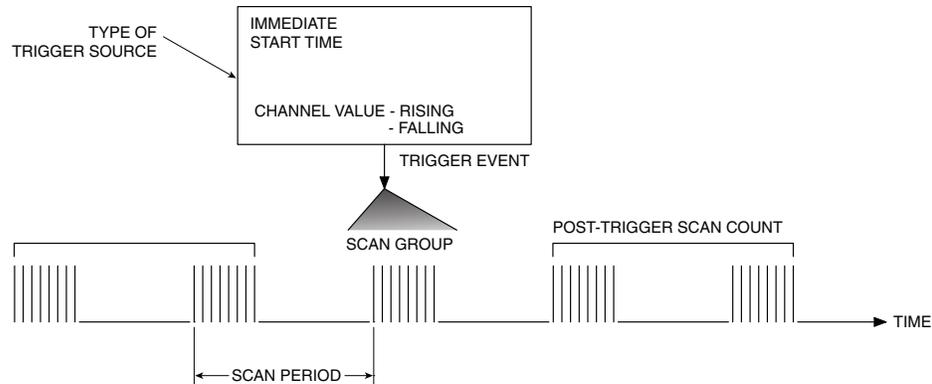
Figure 5-2. Trigger Source Diagram
