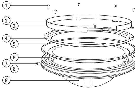
**Figure 3.** Exploded Assembly Diagram, Pendant Lower Dome
