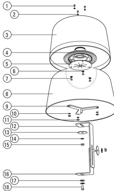
**Figure 1.** Exploded Assembly Diagram, DF8 Pendant Models
