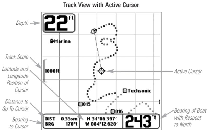
**Panning:** Use the 4-WAY Cursor keys to move the grid around on the display in the direction of the key being pressed. When you do this, a bullseye cursor is drawn at the center of the screen and is linked to the boat by a gray line, even if the boat is off the screen.
