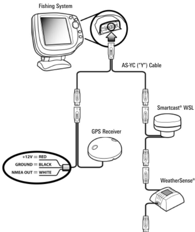
5. The Fishfinder Control Head outputs NMEA signals through the "pigtail" cable attached to the end of the GPS receiver cable for connection to devices such as autopilots. Connect the NMEA Out (White Wire) of the cable to the NMEA In of the device you are connecting to your Fishfinder. The pinouts of this cable are as follows:
