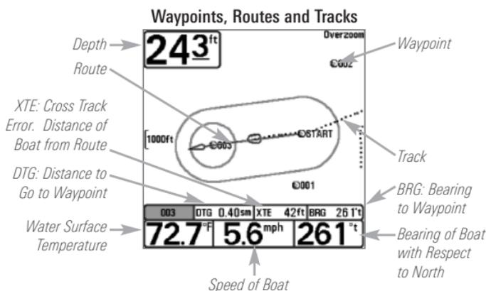
**Routes** link two or more waypoints together to create a path for navigation, and are used in trip planning. A route represents your intended navigation and shows the shortest path from each waypoint to the next. As you travel a route, staying on the route line is the most efficient way to get to your destination, although you should always look out for obstacles not shown on the chart.
