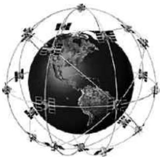
GPS uses a constellation of satellites that continually send radio signals to the earth. Your present position is determined by receiving signals from up to 16 satellites and measuring the distance from the satellites.
