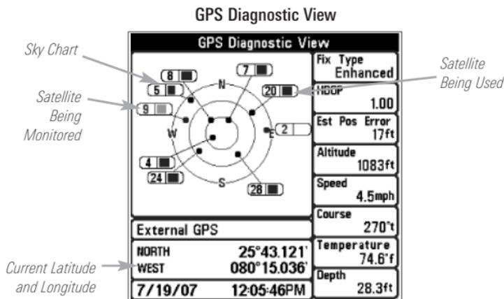
**NOTE:** Units with software versions earlier than 2.54 may require an optional software update to see the satellite data on the satellite status screen and to maximize accuracy from WAAS satellites. This software update is not required for the GPS Receiver to provide normal GPS position, speed, and direction information to your unit.
