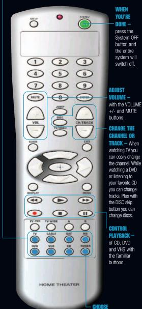
\*\*Make certain to point the remote at the system until the LED stops flashing.
