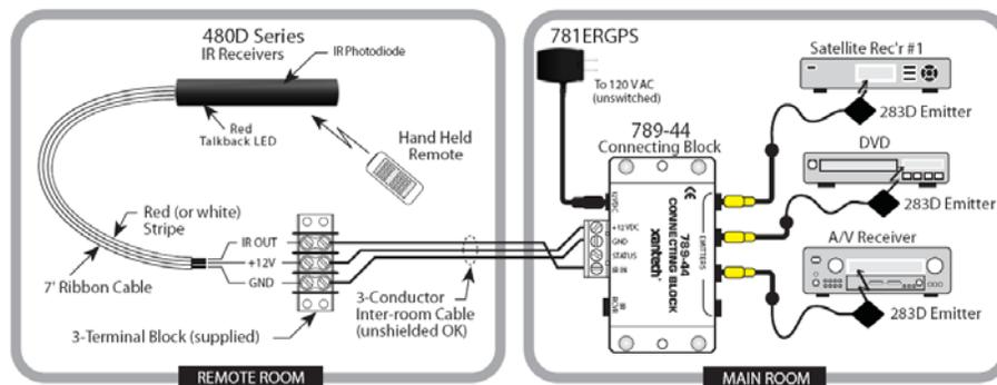
Input connections must be made as illustrated. To extend the emitter wires to a more distant location, you may splice in 2-conductor wire, in the wire gauges mentioned before, as needed.
