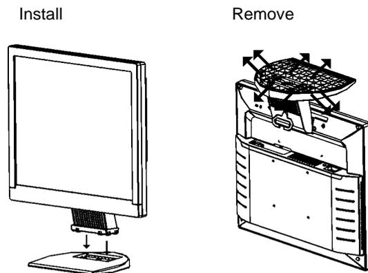
Figure 1 Installing and Removing the Swivel Base
