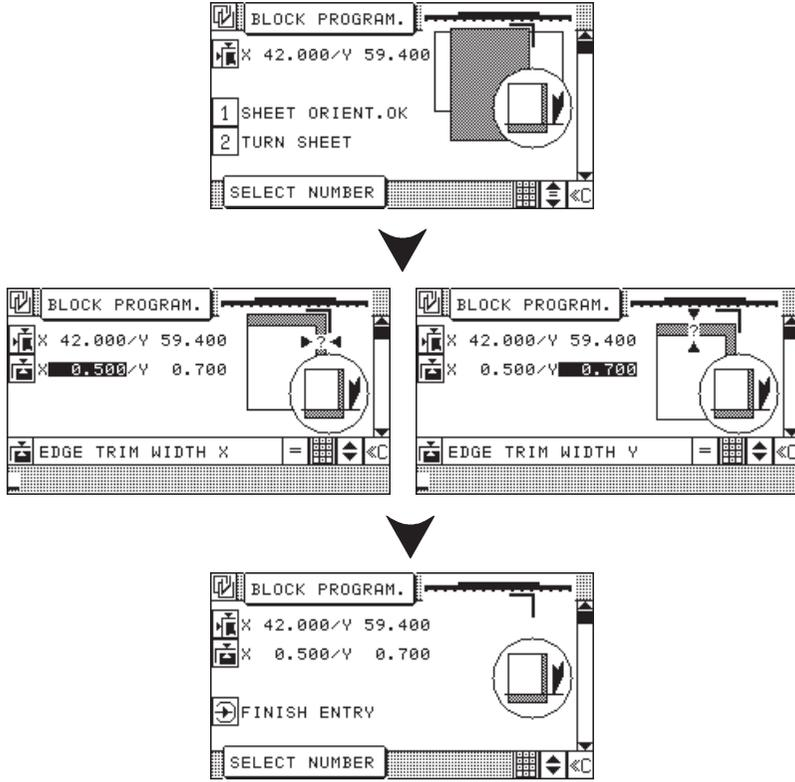
The top screenshot shows the 'BLOCK PROGRAM.' menu with options '1 SHEET ORIENT. OK' and '2 TURN SHEET'. The second screenshot shows the 'EDGE TRIM WIDTH X' parameter being entered. The third screenshot shows the 'EDGE TRIM WIDTH Y' parameter being entered.
