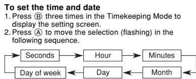
3. While the seconds setting is selected (flashing), press (C) to reset it to 00. If you press (C) while the seconds setting is in the range of 30 to 59, the seconds are reset to 00 and 1 is added to the minutes. If the seconds setting is in the range of 00 to 29, the minutes count is unchanged.
