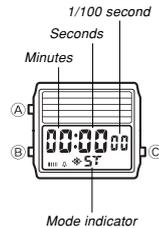
The Stopwatch Mode lets you measure elapsed time, split times, and two finishes. The range of the stopwatch is 59 minutes, 59.99 seconds.
