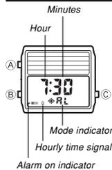
When the Daily Alarm is turned on, the alarm sounds for 20 seconds at the preset time each day. When the Hourly Time Signal is turned on, the watch beeps every hour on the hour.
