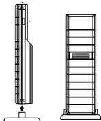
We have provided a mounting plate that you can attach to a surface with the supplied screws. The Sensor can be positioned on a flat surface by securing the stand to the bottom by gently pushing the
