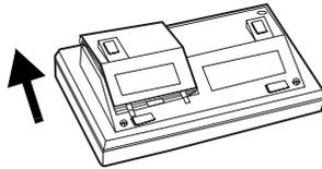
**Caution:** The battery compartment cover is attached to the module. Do not try to remove it completely.
