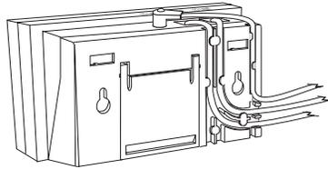
6. Align the keyhole slots on the bracket with the screws in the wall, then slide the module down onto the screws until it is secure.
