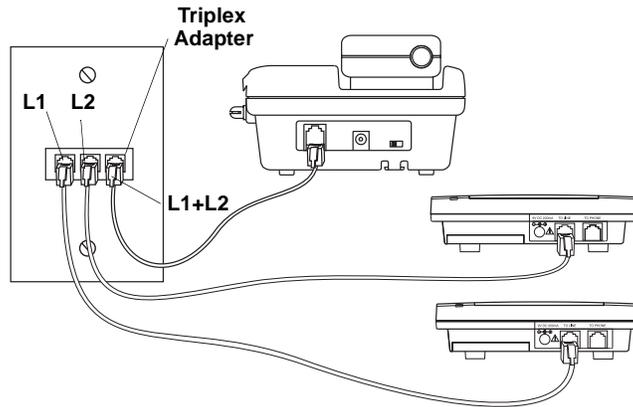
1. Disconnect the telephone line cord from the modular phone jack (on the wall) and plug it into L1+L2 on the triplex adapter.
