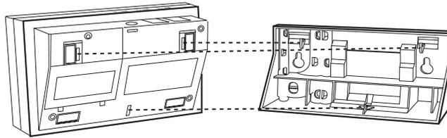
1. Align the slots on the bottom of the module with the hooks on the mounting bracket.
