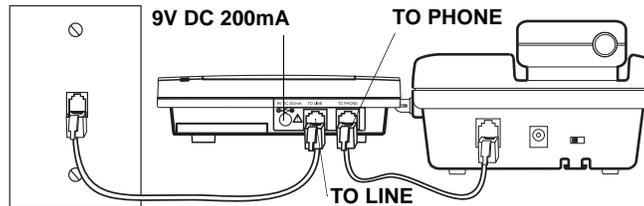
1. Disconnect the telephone line cord from the phone and plug it into the module's **TO LINE** jack.
