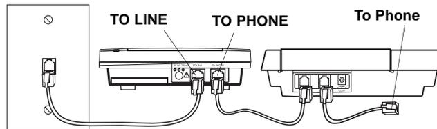
1. Disconnect the phone line cord that connects your answering machine to the phone line from the answering machine's jack. Then plug it into the module's **TO LINE** jack.
