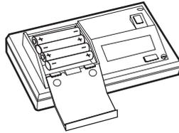
5. Close the cover and secure it with the screw. If you are replacing the batteries, reconnect the phone line, AC adapter, and the phone.
