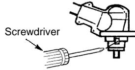
3. While holding the screwdriver in position, remove trimmer head by turning clockwise.
