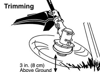
**SCALPING** - The scalping technique removes unwanted vegetation. Hold the bottom of the trimmer head about 3 in. (8 cm) above the ground and at an angle. Allow the tip of the line to strike the ground around trees, posts, monuments, etc. This technique increases line wear.
