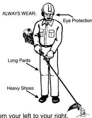
**WARNING:** Always wear eye protection. Never lean over the trimmer head. Rocks or debris can ricochet or be thrown into eyes and face and cause blindness or other serious injury.
