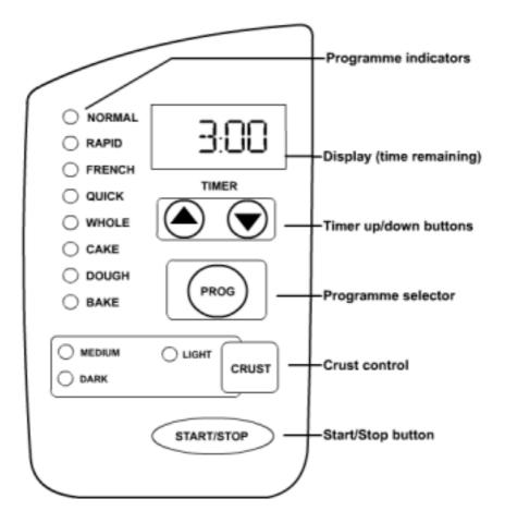
**START/STOP button**. Starts the programme (of course). To stop the programme part way through you need to press and **hold this button for 3 seconds**. After which, the machine will reset to programme 1 (NORMAL).
