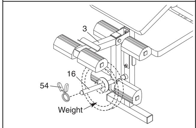
**WARNING:** Do not place more than 150 pounds on the Leg Lever (3) or the Curl Bar (not shown). Use only the Weight Clips (54 or 55) provided with the bench.
