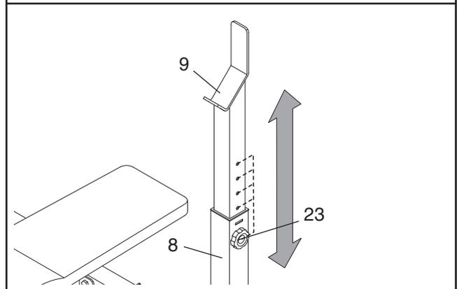
**WARNING:** Always set both Weight Rests (9) at the same height. Make sure the Weight Rest Knobs (23) are inserted into both the Uprights (7, 8) and the Weight Rests.
