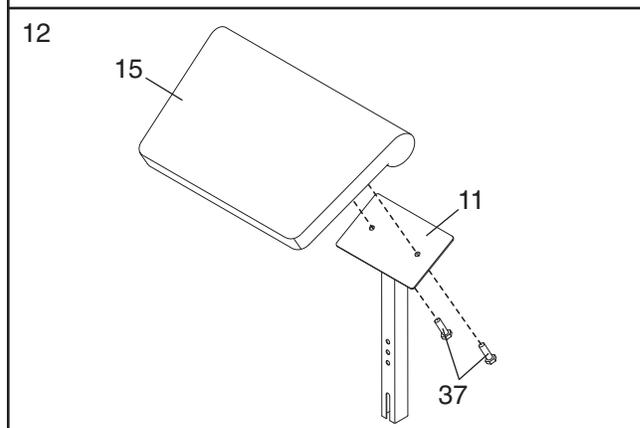
13. **Make sure that all parts are properly tightened before you use the weight bench.** The use of all remaining parts will be explained in ADJUSTMENTS, beginning on the following page.
