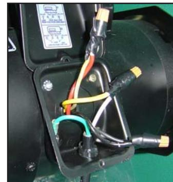
Figure 71. Motor wiring at 220V.
