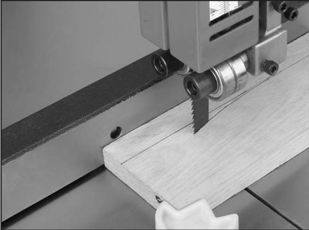
**Figure 61.** Blade leading away from line of cut.
