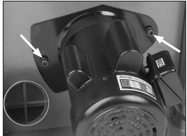
**Figure 43.** Motor mount cap screws.
