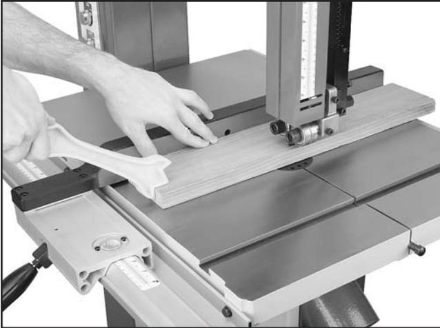
**Figure 39.** Ripping with a push stick.
