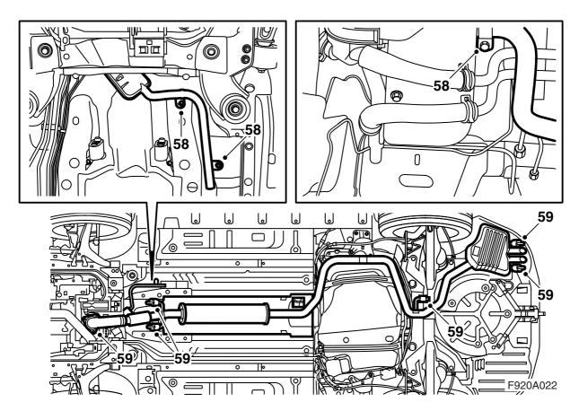
58 Manoeuvre the heater exhaust pipe up towards the heater and fit the end of the pipe onto the exhaust port of the heater. Fasten the exhaust pipe to the floor of the vehicle with the two nuts.
