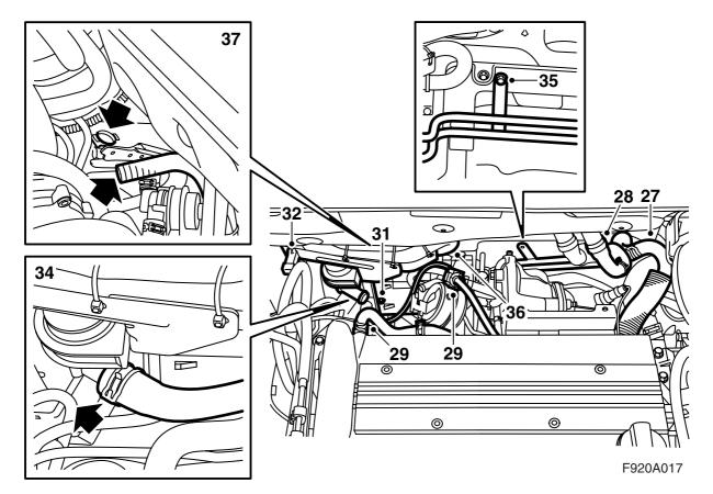
27 Fit the hose clips (including the old clip) onto the new coolant hoses. Connect the hose/pipe assembly between the thermostat housing connection and the heat exchanger connection nearest to the expansion tank. Do not screw the assembly to the bulkhead.
