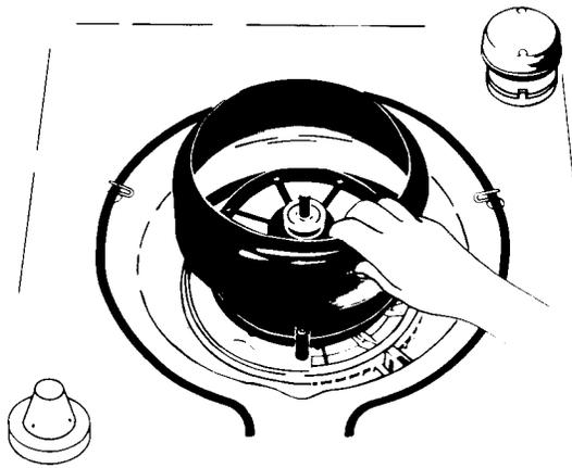
The coarse strainer may be removed, if necessary. To remove, lift strainer out by squeezing center section (F) and remove. To replace, squeeze center section so clips snap into square notch.
