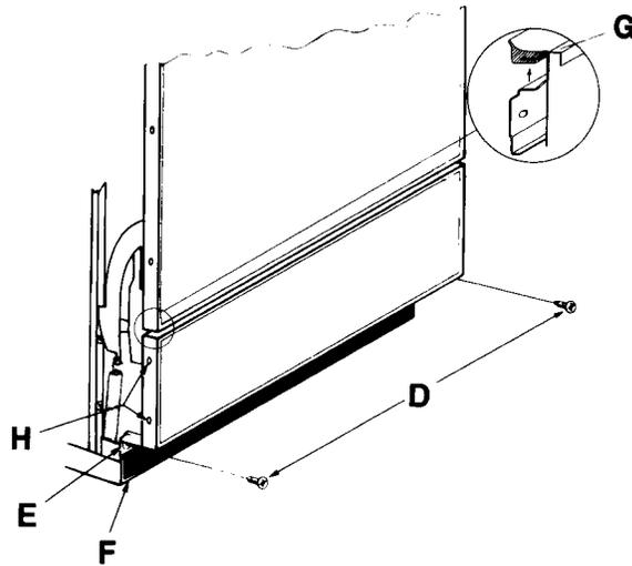
1. Remove two screws (D) located under the access panel.
