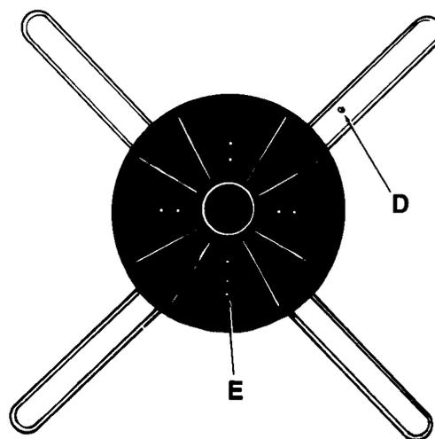
soils remain on the removable filter, lift the 4-Way Hydro Sweep Wash Arm straight up. Check underside of wash arm to make sure the opening of the single stainless steel spray nozzle (D) and the nine water jets (E) are not blocked.
