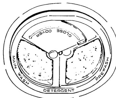
Add detergent to both the Prewash and Main Wash compartments for the Light/China Wash Cycle and the Normal Wash Cycle when dishes are heavily soiled.
