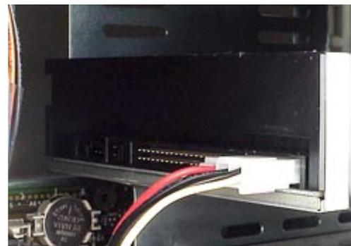
**Figure 4. Installing Power Cable**
