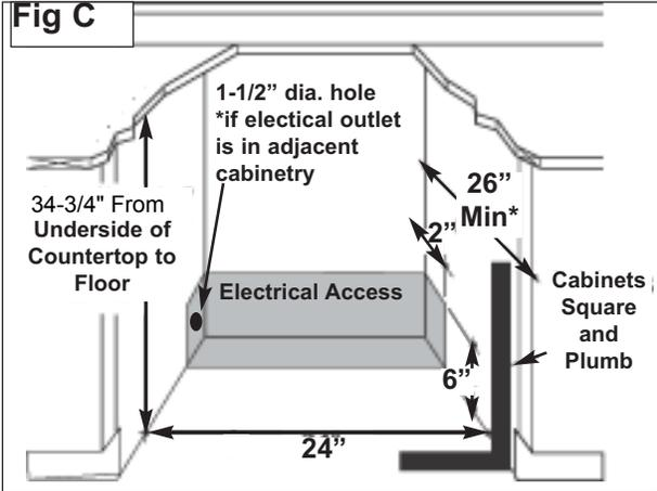
\*The listed depth requirement for the installation is assuming that the electrical outlet is located in the adjacent cabinetry or is flush mounted in the rear wall, not surface mounted in the enclosure.
